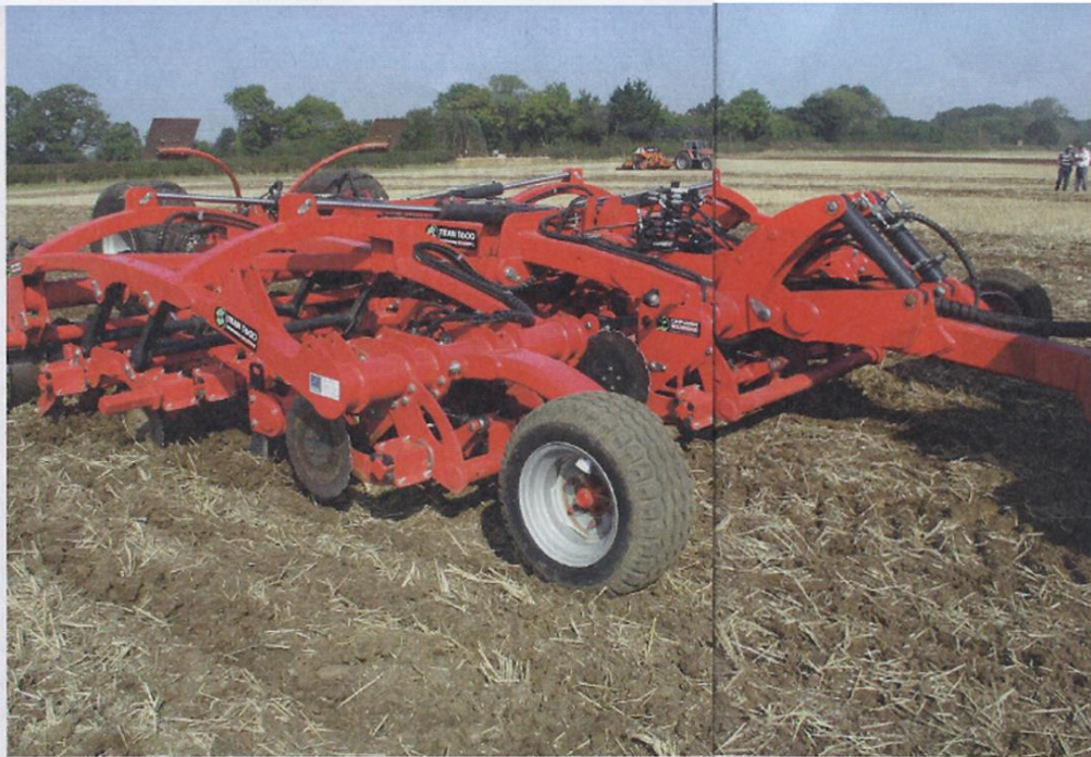
The Titan cultivator has separate push button adjustment of working depth for the tines, which can be adjusted individually
