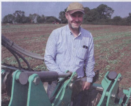
Jim Kelsey demonstrates how the Omni-Lift soil loosener's legs can be lifted out of work individually and held on the quick-release cam-lock mechanism
