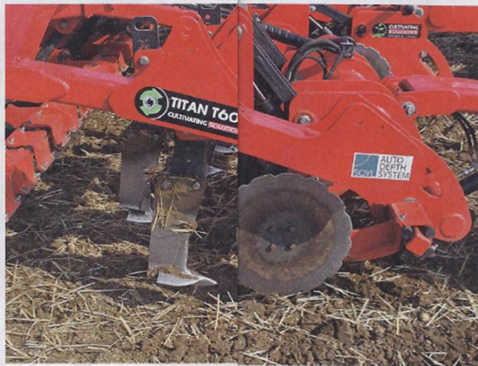
Slim tines on the Titan are designed for minimum surface disturbance
