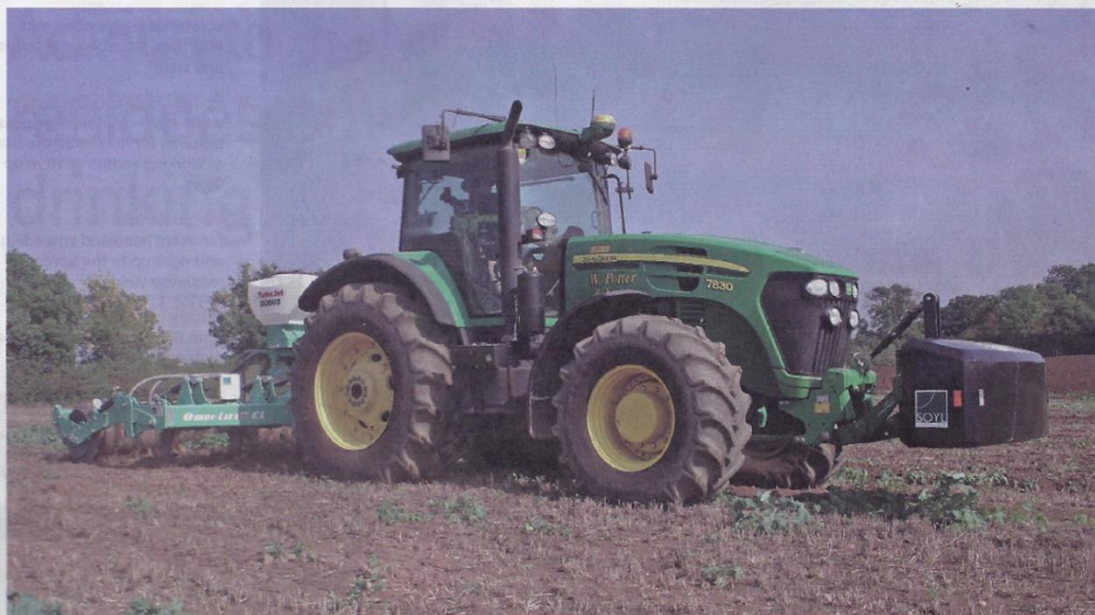
It looks like a conventional front-linkage ballast block, but a closer look reveals a cable between the concrete-encased Topsoil Mapper scan system and the tractor
