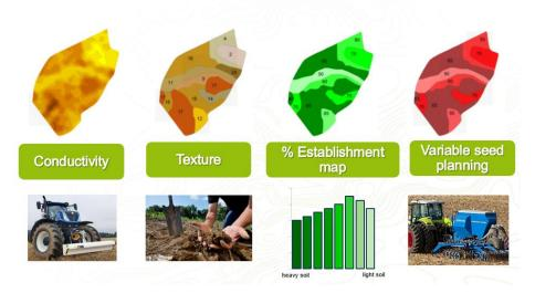
Especially in dry years, this process is key to achieve good yield results. Furthermore, the steering function of the Topsoil Mapper offers us the opportunity to provide a site-specific soil tillage service to our customers. The working depth of the implement is automatically adapted to the actual soil conditions (deeper/flatter). That saves diesel and time and reduces machine wear, without reducing the effect of tillage.
